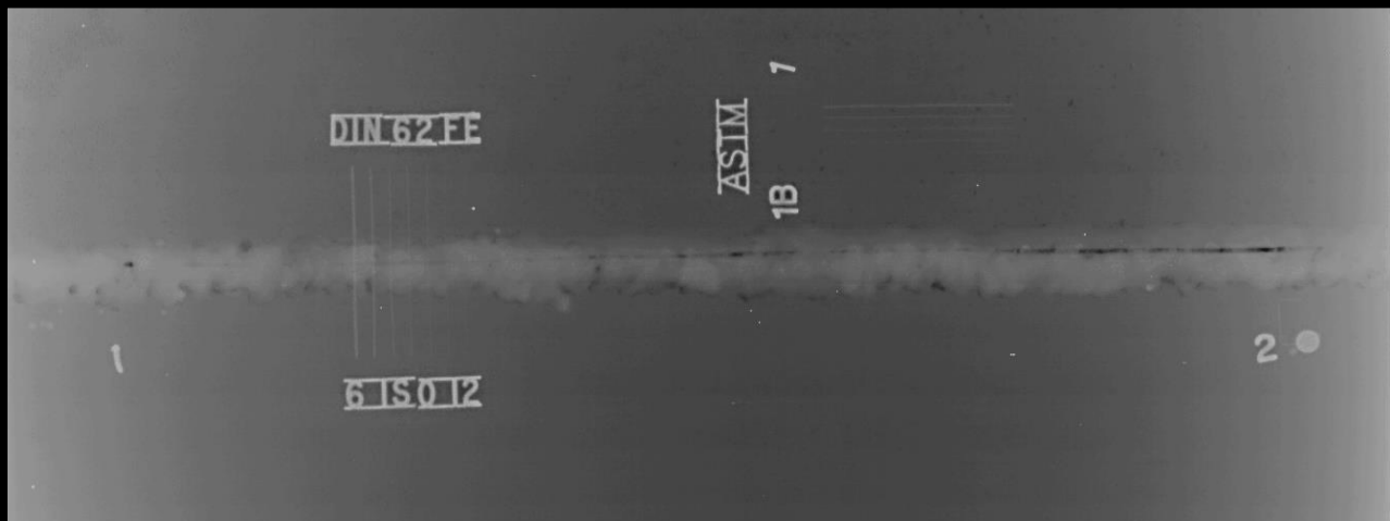
15mm Plate Vertical weld with significant incomplete penetration, undercut and porosity. Shown in Raw acquisition format with no image enhancement.
